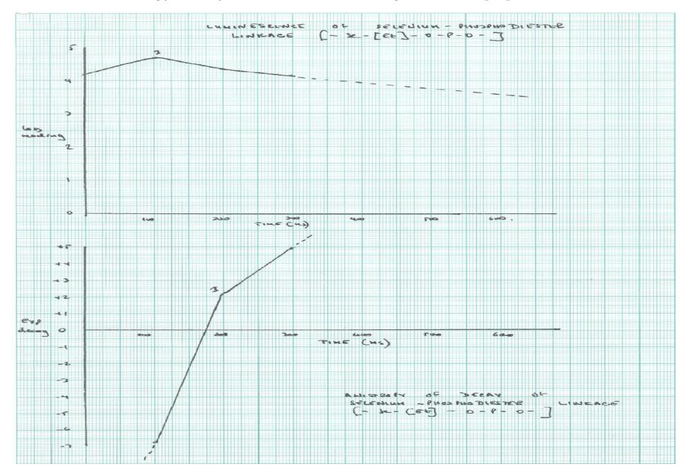
Emission energy decay of PL and LPL linkages with Se-O-P-O structure.
