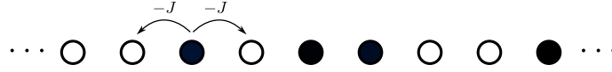
Figure 1: Illustration of a one-dimensional lattice on which fermions can hop with amplitude -J . Note that hopping is constrained because no two fermions can occupy the same lattice site due to the Pauli exclusion principle.
